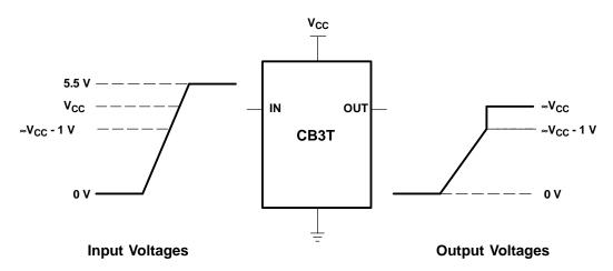
If the input high voltage ( $V_{IH}$ ) level is greater than or equal to  $V_{CC}$  - 1 V, and less than or equal to 5.5 V, the output high voltage ( $V_{OH}$ ) level will be equal to approximately the  $V_{CC}$  voltage level.
