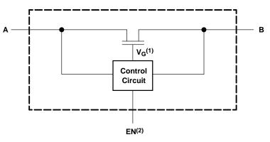
(1) Gate voltage (V<sub>G</sub>) is equal to approximately  $V_{CC} + V_T$  when the switch is ON and  $V_I > V_{CC} + V_T$ .
