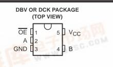
This device is fully specified for partial-power-down applications using I<sub>off</sub>. The I<sub>off</sub> feature ensures that damaging current will not backflow through the device when it is powered down. The device has isolation during power off.
