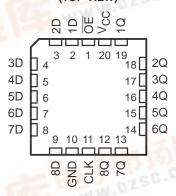
A buffered output-enable ( $\overline{OE}$ ) input places the eight outputs in either a normal logic state (high or low) or the high-impedance state. In the high-impedance state, the outputs neither load nor drive the bus lines significantly. The high-impedance state and the increased drive provide the capability to drive bus lines without interface or pullup components.
