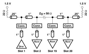
Figure 2. High-Drive Test Backplane
