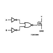
Fig.5 Logic diagram (one gate).
