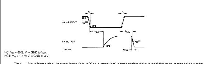
Fig.6 Waveforms showing the input (nA, nB) to output (nY) propagation delays and the output transition times.
