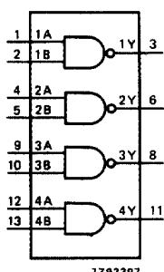
Fig.4 Functional diagram.
