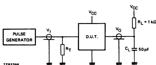
Fig.7 Test circuit (open drain)
