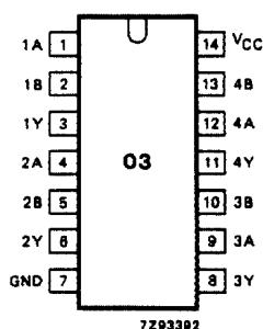
Fig.1 Pin configuration.
