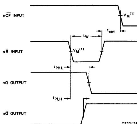
Fig.7 Waveforms showing the reset ( $n\bar{R}$ ) input to output ( $nQ$ ,  $n\bar{Q}$ ) propagation delays, the reset pulse width and the  $n\bar{R}$  to  $n\bar{C}P$  removal time.
