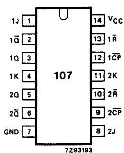
Fig.1 Pin configuration.
