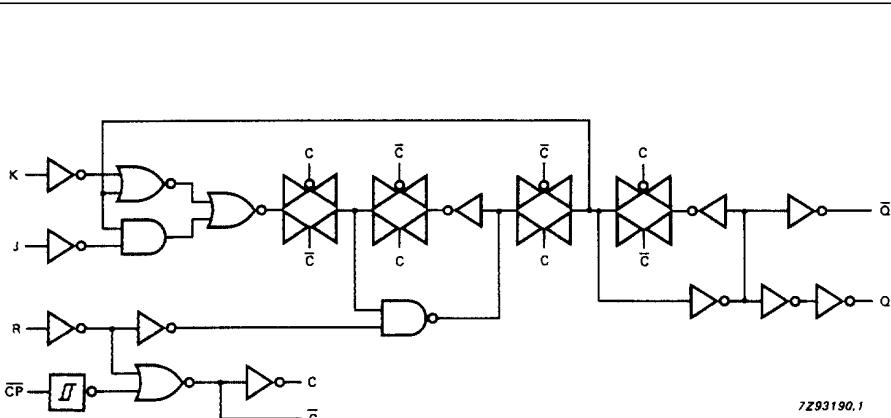
Fig.5 Logic diagram (one flip-flop).
