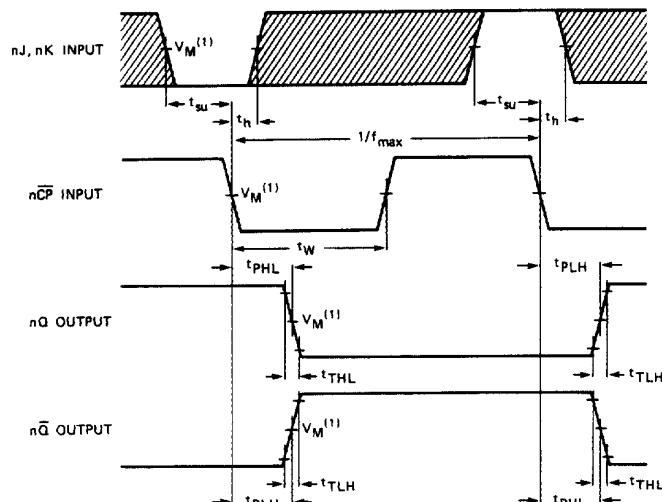
Fig.6 Waveforms showing the clock ( $n\bar{C}P$ ) to output ( $nQ$ ,  $n\bar{Q}$ ) propagation delays, the clock pulse width, the J and K to  $n\bar{C}P$  set-up and hold times, the output transition times and the maximum clock pulse frequency.
