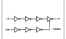
Fig.5 Logic diagram (one buffer).
