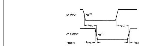
(1) HC :  $V_M$  = 50%;  $V_I$  = GND to  $V_{CC}$ . HCT:  $V_M$  = 1.3 V;  $V_I$  = GND to 3 V.
