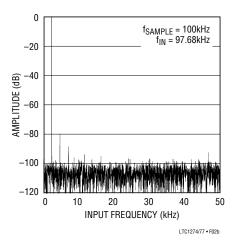
Figure 2b. LTC1274 Nonaveraged, 4096 Point FFT Plot with 100kHz Input Frequency
