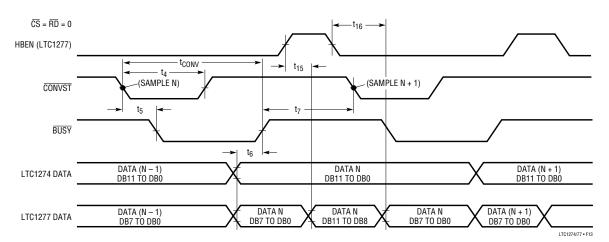
Figure 13. Mode 1a. CONVST Starts a Conversion. Data Outputs Always Enabled  $(\overline{\text{CONVST}} = \sqrt[3]{1})$
