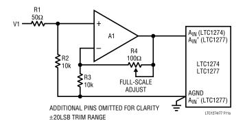
Figure 11a. Full-Scale Adjust Circuit
