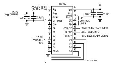
Figure 9. LTC1274 Typical Circuit
