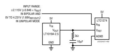
Figure 7. Supplying a 2.5V Reference Voltage to the LTC1274 with the LT1019A-2.5
