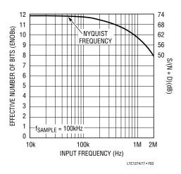
Figure 3. ENOBs and S/(N + D) vs Input Frequency
