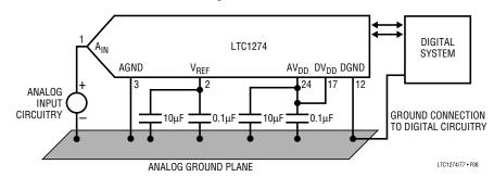
Figure 8. Power Supply Grounding Practice
