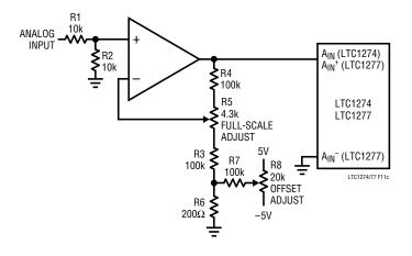
Figure 11c. LTC1274/LTC1277 Bipolar Offset and Full-Scale Adjust Circuit
