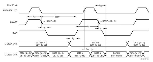
Figure 14. Mode 1b.  $\overline{\text{CONVST}}$  Starts a Conversion. Data Outputs Always Enabled  $(\overline{\text{CONVST}} = \boxed{?}$
