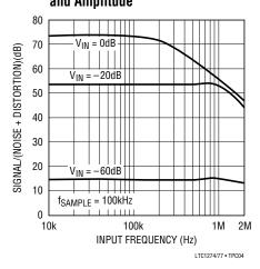
Signal-to-Noise Ratio (Without Harmonics) vs Input Frequency
