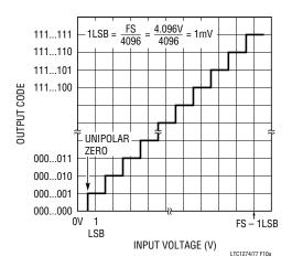
Figure 10a. LTC1274/LTC1277 Unipolar Transfer Characteristics
