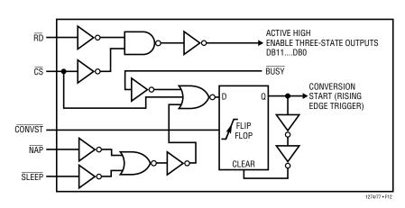
Figure 12. Internal Logic for Control Inputs CS, RD, CONVST, NAP and SLEEP (LTC1277)
