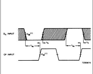
The shaded areas indicate when the input is permitted to change for predictable output performance.
