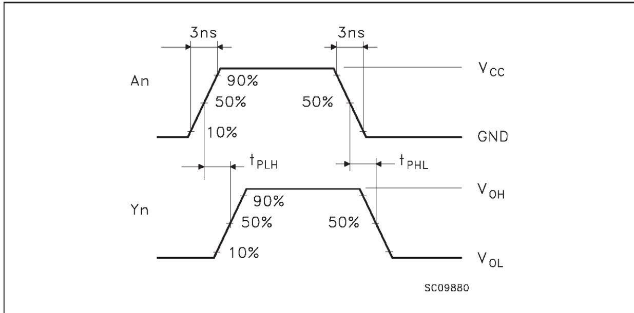
**WAVEFORM 2: OUTPUT ENABLE AND DISABLE TIME** ( $f=1\text{MHz}$ ; 50% duty cycle)
