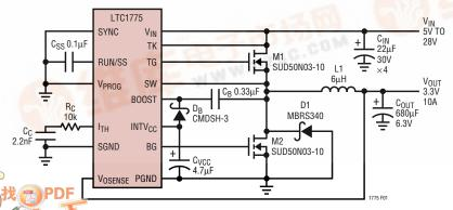
Figure 1. High Efficiency Step-Down Converter
