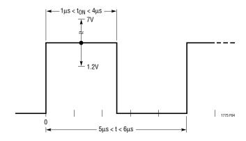
Figure 4. SYNC Clock Waveform
