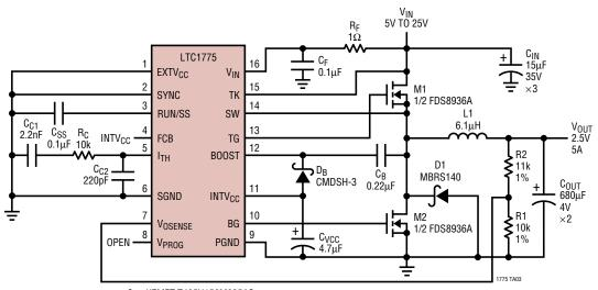
C<sub>IN</sub>: KEMET T495X156M035AS C<sub>OUT</sub>: KEMET T510X687K004AS L1: SUMIDA CDRH127-6R1
