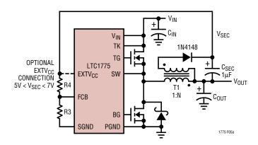
Figure 5a: Secondary Output Loop and EXTV<sub>CC</sub> Connection
