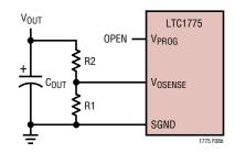
Figure 8b. Adjustable V<sub>OUT</sub>
