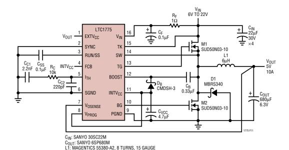
Figure 11. 5V/10A Fixed Output from Design Example
