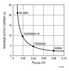
Figure 3. Maximum Output Current vs  $R_{DS(ON)}$  at  $V_{GS} = 4.5V$
