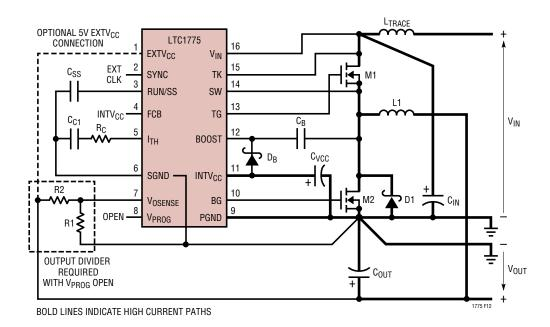
Figure 12. LTC1775 Layout Diagram
