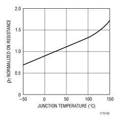
Figure 2. R<sub>DS(ON)</sub> vs Temperature
