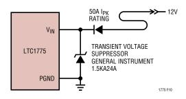
Figure 10. Automotive Application Protection
