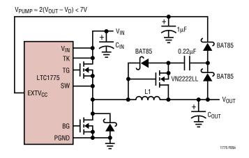
Figure 5b: Capacitive Charge Pump for EXTV<sub>CC</sub>
