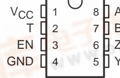
SN75178B . . . P PACKAGE (TOP VIEW)
