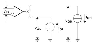
Figure 2. Receiver Test Circuit, VOH and VOL
