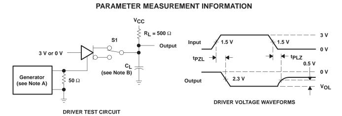
NOTES: A. The pulse generator has the following characteristics: PRR  $\leq$  1 MHz, 50% duty cycle, t<sub>f</sub>  $\leq$  10 ns, t<sub>f</sub>  $\leq$  10 ns. B. C<sub>1</sub> includes probe and jig capacitance.
