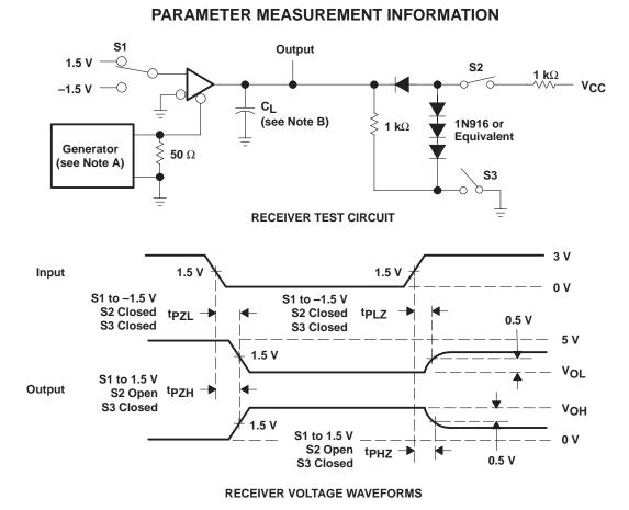
NOTES: A. The pulse generator has the following characteristics: PRR  $\leq$  1 MHz, 50% duty cycle, t<sub>f</sub>  $\leq$  10 ns. t<sub>f</sub>  $\leq$  10 ns. B. C<sub>L</sub> includes probe and jig capacitance.
