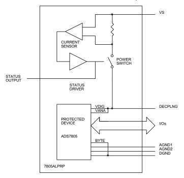
FIGURE 3. LATCHUP PROTECTION DIAGRAM
