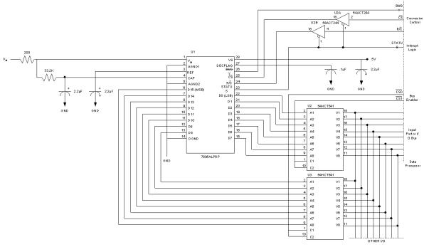
FIGURE 6. TYPICAL 7805A CIRCUIT WITH 8-BIT BUS INTERFACE
