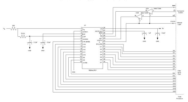
FIGURE 5. TYPICAL 7805A CIRCUIT WITH 16-BIT BUS INTERFACE
