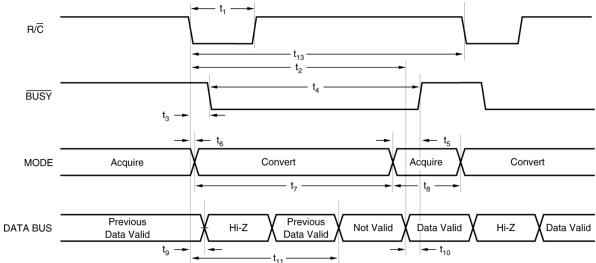
FIGURE 2. USING CS TO CONTROL CONVERSION AND READ TIMING
