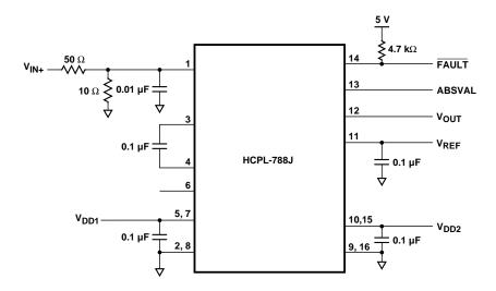
Figure 20. AC Test Circuit.
