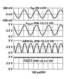
Figure 19. Sine Response 400 mV pk to pk 4 kHz Input, at  $V_{\rm REF}$  = 5 V.
