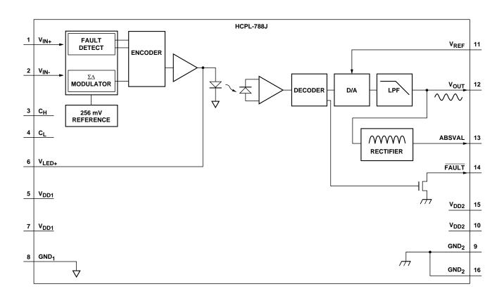
Figure 21. Internal Block Diagram.
