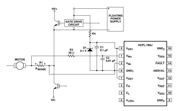
Figure 26. Recommended Supply and Sense Resistor Connections.
