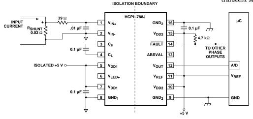
Figure 1. Current Sensing Circuit.
