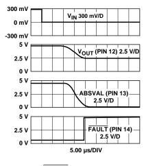
Figure 16.  $\overline{FAULT}$  Release, 300 to 0 mV Input, at  $V_{REF} = 5$  V.
