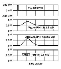
Figure 17.  $\overline{FAULT}$  Rejecting a 1  $\mu s$ , 0 to 2 V to 0 Input. Rejection is Independent of Amplitude.
