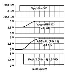
Figure 15.  $\overline{FAULT}$  Detection, 0 to 300 mV Input, at  $V_{REF} = 5 \text{ V}$ .
