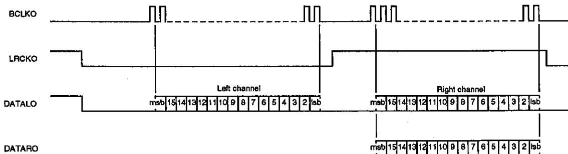
Figure 10. Four-times oversampling, format B output data format
