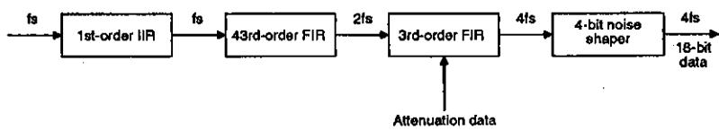
Figure 2. Double-rate mode eight-times oversampling filter
