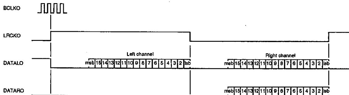
Figure 8. Four-times oversampling, format A output data format
