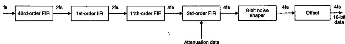
Figure 3. Normal-rate mode four-times oversampling filter
