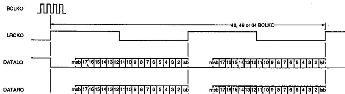
Figure 7. Eight-times oversampling, format A output data format
