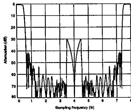
**Normal-rate mode with four-times oversampling**
