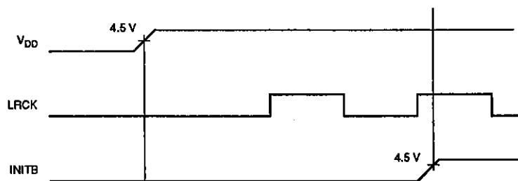
Figure 5. Initialization waveform
