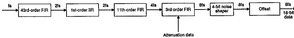
Figure 1. Normal-rate mode eight-times oversampling filter
