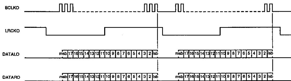
Figure 9. Eight-times oversampling, format B output data format
