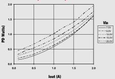
Note 1: All data listed in the above graphs, except for derating data, has been developed from actual products tested at 25°C. This data is considered typical data for the ISR. Note 2: Thermal derating graphs are developed in free air convection cooling of 40-60 LFM. (See Thermal Application Note)
