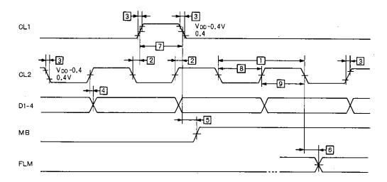
Ta = -20 to + 75 °C, VDD = 5 V = 5 %, GND = 0 V
