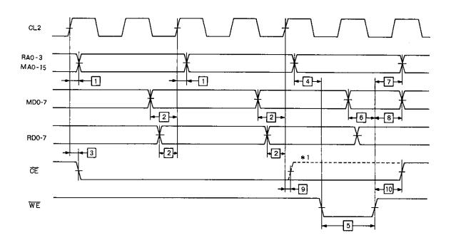
READ CYCLE (Ta=-20 to +75°C, VDD=5 V $\pm$  5%, GND=0 V)
