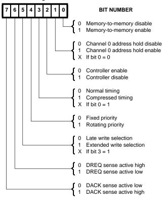
**Mode Register** - Each channel has a 6-bit Mode register associated with it. When the register is being written to by the microprocessor in the Program condition, bits 0 and 1 determine which channel Mode register is to be written. When the processor reads a Mode register, bits 0 and 1 will both be ones. See the following diagram and Figure 4 for Mode register functions and addresses.
