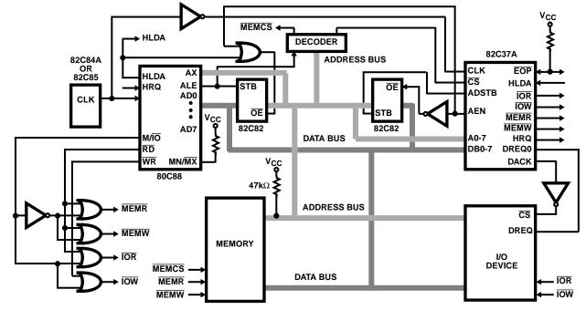
NOTE: The address lines need pull-up resistors.
