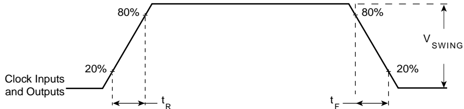
FIGURE 6 - INPUT AND OUTPUT RISE AND FALL TIME
