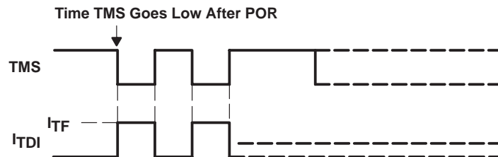
Figure 6. Fuse Check Mode Current, MSP430C33xA
