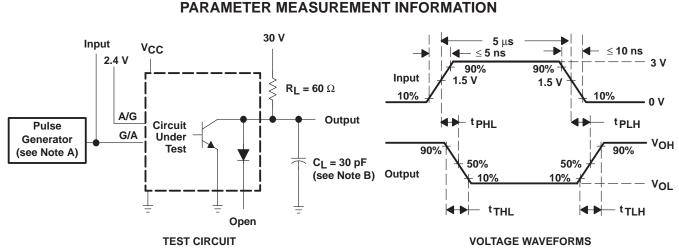
NOTES: A. The pulse generator has the following characteristics: PRR = 100 kHz,  $Z_0$  = 50  $\Omega$ . B. C<sub>L</sub> includes probe and jig capacitance.
