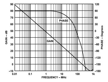
Figure 41. Open-Loop Frequency Response
