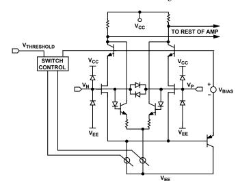
Figure 45. Simplified Input Schematic
