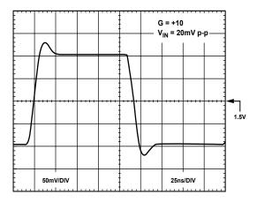
Figure 16. Small Signal Transient Response 5 V Supply
