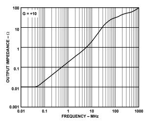
Figure 28. Output Impedance vs. Frequency
