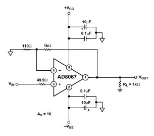
Figure 34. Standard Test Circuit
