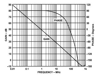
Figure 13. Open-Loop Gain and Phase
