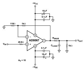
Figure 36. Test Circuit for Capacitive Load
