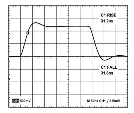
Figure 53. Photodiode Preamplifier Pulse Response
