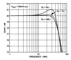
Figure 10. Small Signal Frequency Response for Various R<sub>F</sub>
