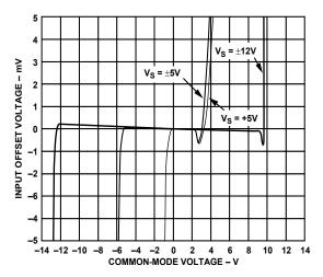
Figure 26. Input Offset Voltage vs. Common-Mode Voltage
