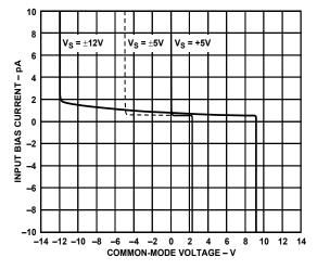
Figure 25. Input Bias Current vs. Common-Mode Voltage
