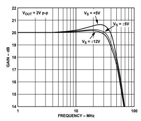
Figure 6. Large Signal Frequency Response for Various Supplies
