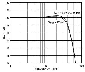
Figure 9. Frequency Response for Various Output Amplitudes
