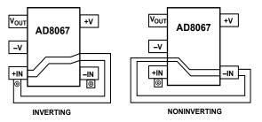
Figure 48. Guard-Ring Layout SOT-23-5
