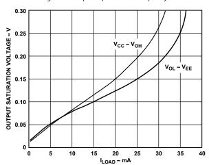
Figure 29. Output Saturation Voltage vs. Output Load Current
