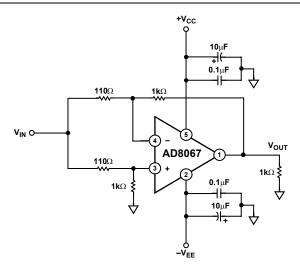
Figure 37. CMRR Test Circuit
