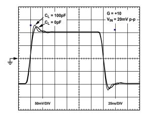
Figure 19. Small Signal Transient Response  $\pm$  5 V Supply
