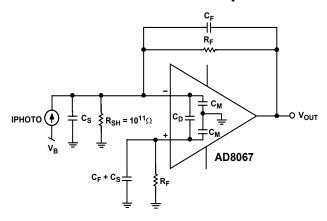
Figure 49. Wideband Photodiode Preamp
