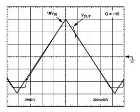
Figure 17. Output Overdrive Recovery
