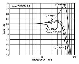
Figure 8. Small Signal Frequency Response for Various CLOAD
