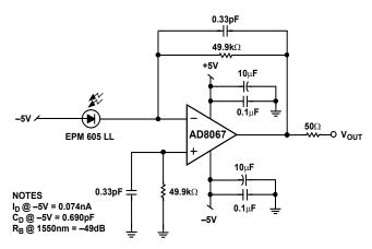
Figure 51. Photodiode Preamplifier
