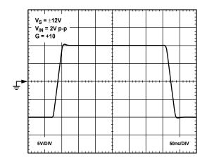
Figure 20. Large Signal Transient Response
