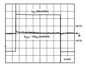
Figure 18. Long-Term Settling Time
