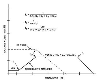
Figure 50. Photodiode Voltage Noise Contributions
