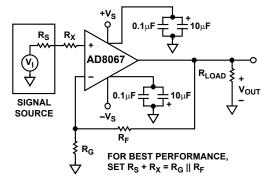
Figure 40. Noninverting Gain Configuration
