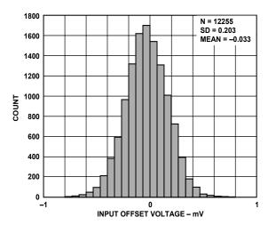
Figure 23. Input Offset Voltage Histogram
