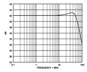
Figure 58. Gain Bandwidth Response
