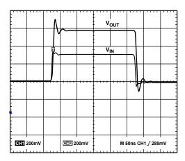
Figure 55. Gain of 2 Pulse Response
