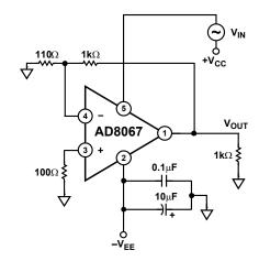
Figure 38. Positive PSRR Test Circuit
