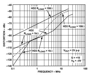
Figure 11. Distortion vs. Frequency for Various Loads
