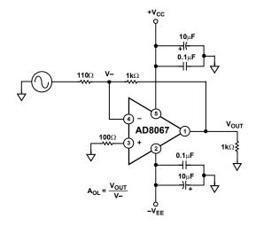
Figure 35. Open-Loop Gain Test Circuit
