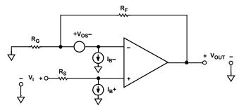
Figure 44. Op Amp DC Error Sources
