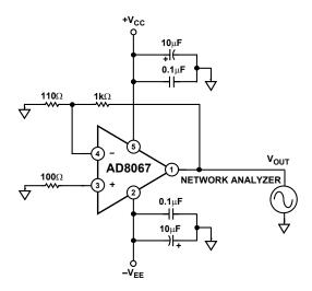
Figure 39. Output Impedance Test Circuit
