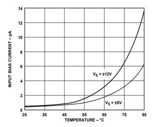
Figure 22. Input Bias Current vs. Temperature
