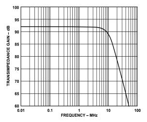
Figure 52. Photodiode Preamplifier Frequency Response
