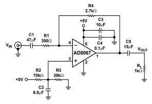
Figure 56. Single-Supply Operation Schematic
