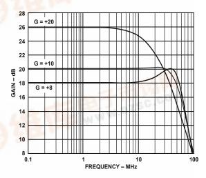
Figure 2. Small Signal Frequency Response
