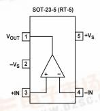
Figure 1. Connection Diagram (Top View)
