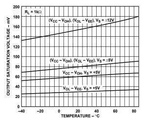
Figure 32. Output Saturation Voltage vs. Temperature
