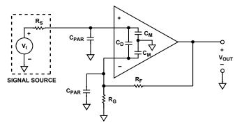
Figure 43. Input and Board Capacitances
