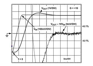
Figure 21. 0.1% Short-Term Settling Time
