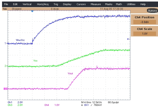
Figure 15 - Start up waveforms Ch1: V_{in}=V_{cc} , Ch3: V_{ss} , Ch4: V_{out}
