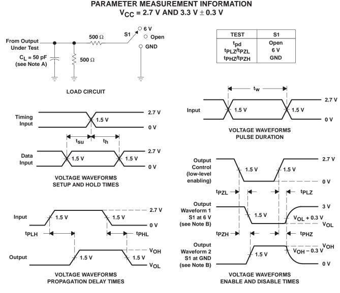
NOTES: A.  $\ensuremath{\mathsf{C}}_L$  includes probe and jig capacitance.
