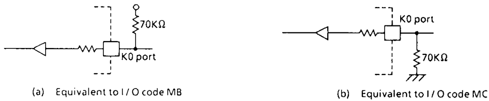
Figure 1-2. I/O code and external circuitry
