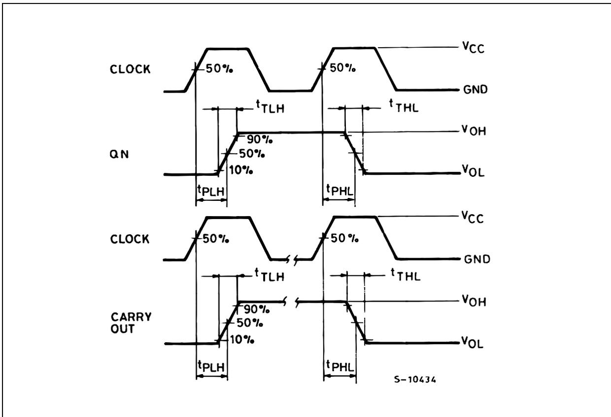
WAVEFORM 2 : MINIMUM SETUP AND HOLD TIME (f=1MHz; 50% duty cycle)
