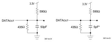
Figure 1 AC Output Test Load
