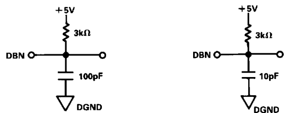
a. High-Z to V OL b. V OL to High-Z Figure 5. Load Circuit for \overline{\text{INT}} Propagation Delays
