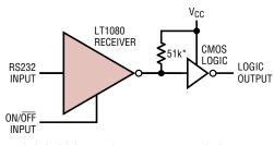
\* FORCES LOGIC INPUT STATE WHEN V<sub>ON/OFF</sub> IS LOW 1080/81 F0
