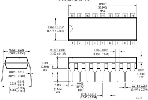
\*THESE DIMENSIONS DO NOT INCLUDE MOLD FLASH OR PROTRUSIONS.
