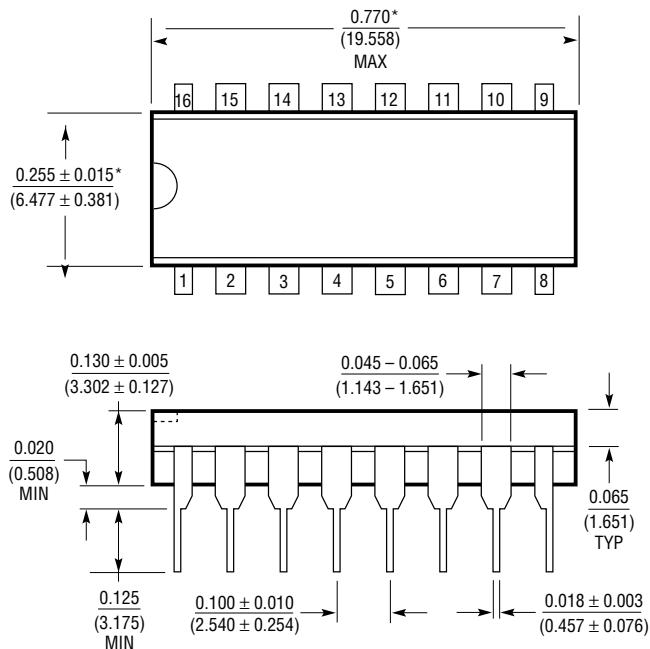
\*THESE DIMENSIONS DO NOT INCLUDE MOLD FLASH OR PROTRUSIONS.
