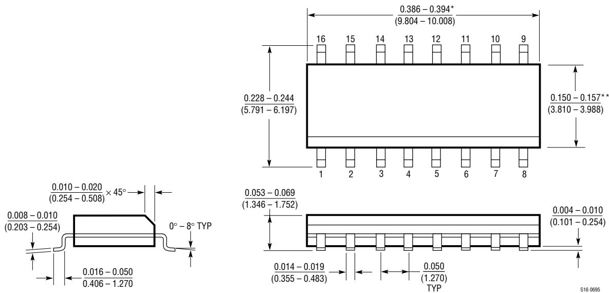
\*DIMENSION DOES NOT INCLUDE MOLD FLASH. MOLD FLASH
