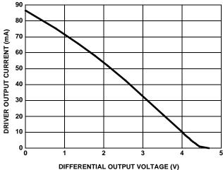
FIGURE 6. DRIVER OUTPUT CURRENT vs DIFFERENTIAL
