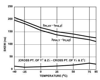
FIGURE 11. DRIVER SKEW vs TEMPERATURE (ISL8487, ISL81483)
