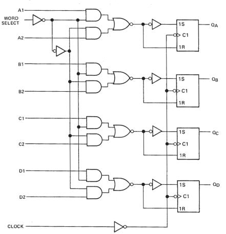
schematics of inputs and outputs
