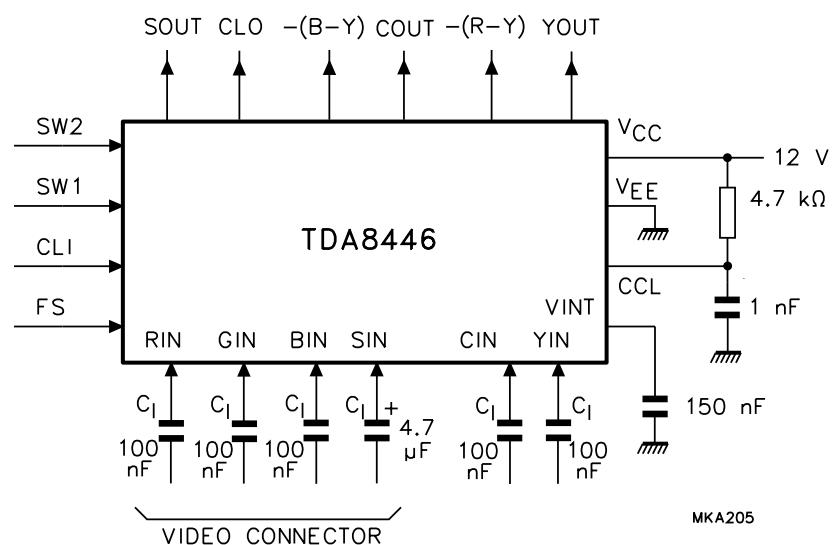
Fig.5 Typical application circuit.
