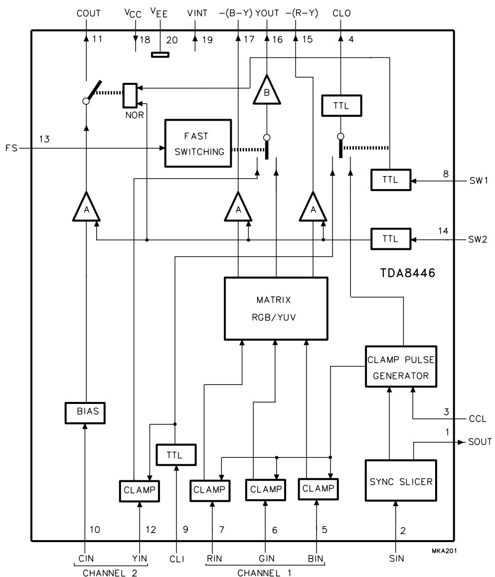
Fig.1 Block diagram (TDA8446).
