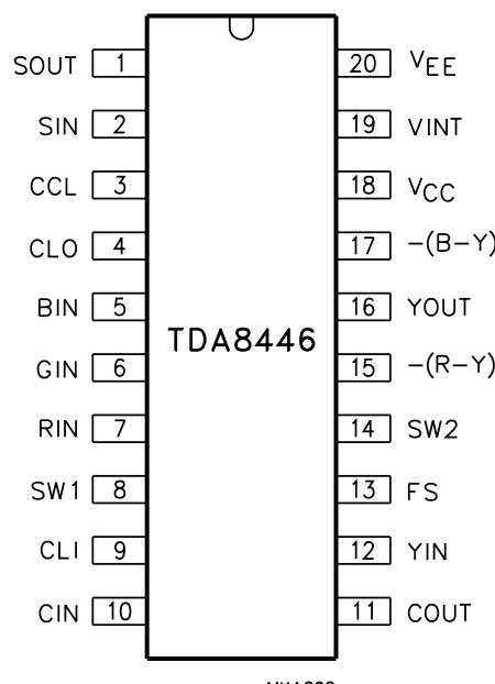
Fig.2 Pin configuration (DIP20).
