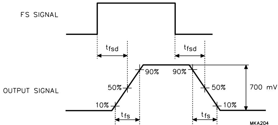
Fig.4 Fast switching times.
