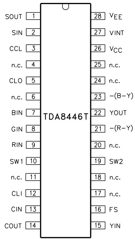
Fig.3 Pin configuration (SO28).
