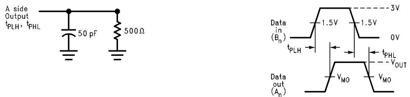
FIGURE 3. B to A Direction Test Load and Waveforms for Outputs A 1 - A 4
