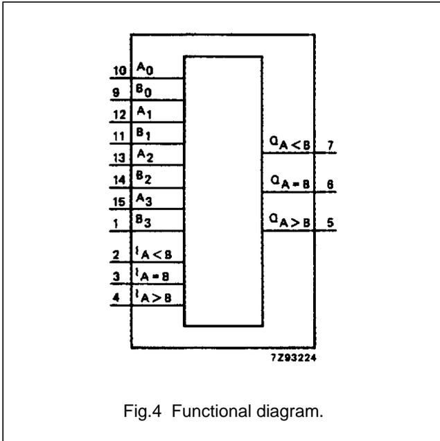
Fig.4 Functional diagram.
