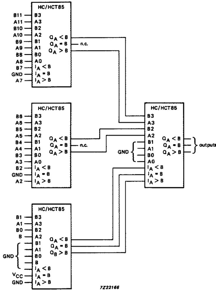
Fig.8 Parallel cascading; comparing 12-bit words.
