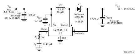
FIGURE 33. +5V to +12V Boost Regulator
