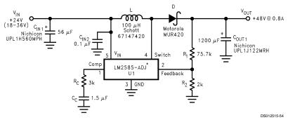
\*The LM2585 will require a heat sink in these applications. The size of the heat sink will depend on the maximum ambient temperature. To calculate the thermal resistance of the IC and the size of the heat sink needed, see the "Heat Sink/Thermal Considerations" section in the Application Hints.
