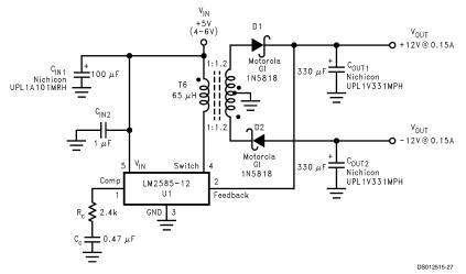
FIGURE 10. Dual-Output Flyback Regulator
