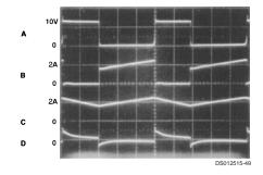
A: Switch Voltage, 10 V/div B: Switch Current, 2 A/div C: Inductor Current, 2 A/div D: Output Ripple Voltage, 100 mV/div, AC-Coupled Horizontal: 2 µs/div
