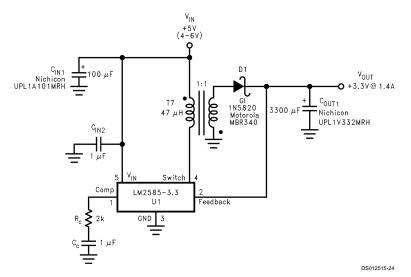
FIGURE 7. Single-Output Flyback Regulator
