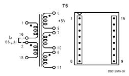
Top View FIGURE 23. Pulse PE-68413 (Surface Mount)
