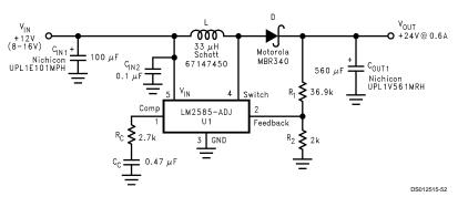
FIGURE 35. +12V to +24V Boost Regulator
