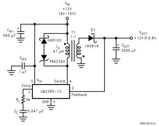
As shown in Figure 4, the LM2585 can be used as a flyback regulator by using a minimum number of external components. The switching waveforms of this regulator are shown in Figure 5. Typical Performance Characteristics observed during the operation of this circuit are shown in Figure 6.
