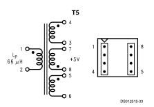
Top View FIGURE 18. Coilcraft Q4338-B
