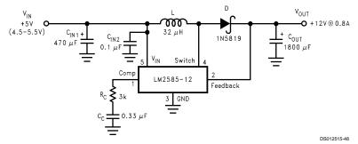
By adding a small number of external components (as shown in Figure 30), the LM2585 can be used to produce a regulated output voltage that is greater than the applied input voltage. The switching waveforms observed during the operation of this circuit are shown in Figure 31. Typical performance of this regulator is shown in Figure 32.
