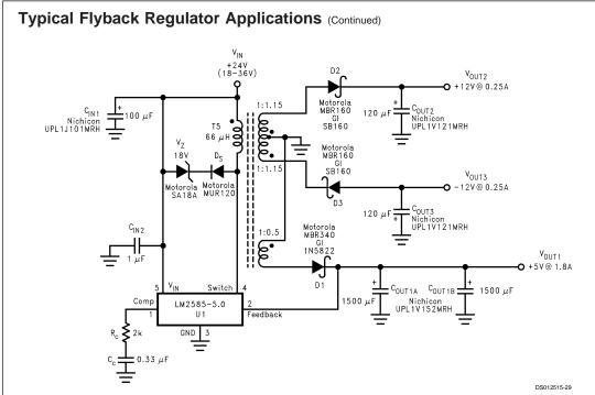
FIGURE 12. Triple-Output Flyback Regulator
