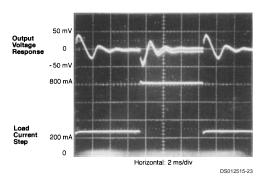
FIGURE 6. V<sub>OUT</sub> Load Current Step Response
