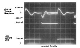
FIGURE 32. V<sub>OUT</sub> Response to Load Current Step
