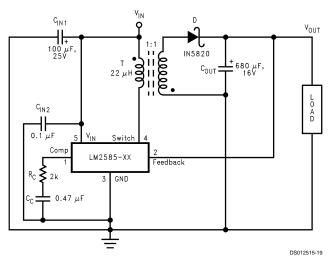
$C_{IN1}-100~\mu F,$  25V Aluminum Electrolytic  $C_{IN2}-0.1~\mu F$  Ceramic  $T-22~\mu H,$  1:1 Schott #67141450 D-1N5820
