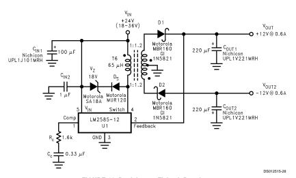
FIGURE 11. Dual-Output Flyback Regulator
