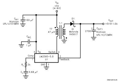
FIGURE 8. Single-Output Flyback Regulator
