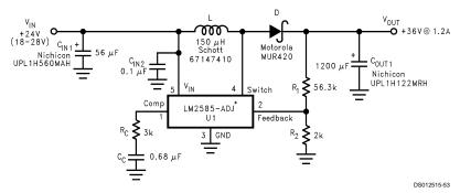
FIGURE 36. +24V to +36V Boost Regulator
