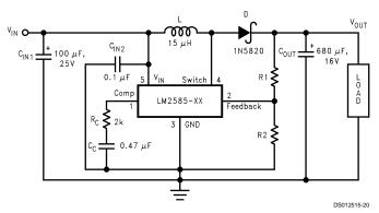
$C_{\text{IN1}}$  — 100  $\mu\text{F}$ , 25V Aluminum Electrolytic
