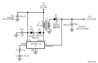
FIGURE 9. Single-Output Flyback Regulator
