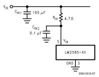
FIGURE 40. Input Line Filter
