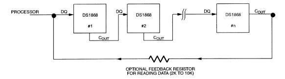
The C<sub>OUT</sub> output of the DS1868 can be used to drive the DQ input of another DS1868. When connecting multiple devices, the total number of bits transmitted is always 17 times the number of DS1868s in the daisy chain.
