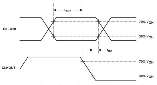
Figure 6. Setup and Hold Time Waveforms
