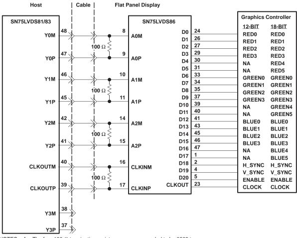
NOTES: A. The four 100- $\Omega$  terminating resistors are recommended to be 0603 types.
