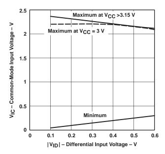
Figure 3. Maximum Common-Mode Input Voltage Vs Differential Input Voltage and  $V_{\hbox{\scriptsize CC}}$
