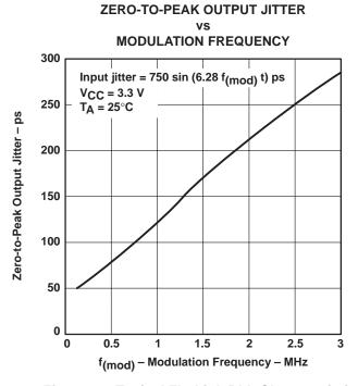
Figure 12. Typical FlatLink PLL Characteristics
