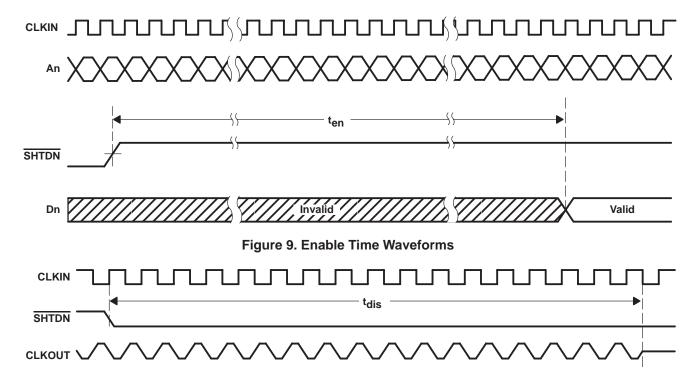
Figure 10. Disable Time Waveforms
