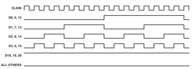
NOTE A: The 16-grayscale test-pattern test device power consumption for a typical display pattern.
