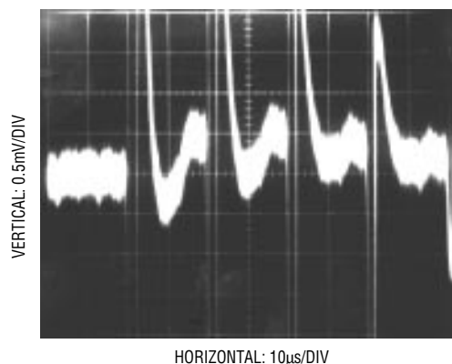
Figure 14. Poor Reference Settling Can Cause A/D Errors
