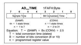
The converter is ratiometric, so absolute accuracy is dependent on the accuracy and stability of  $V_{REF}$ .  $V_{REF}$  must be close to  $V_{CC}$  since it supplies both the resistor ladder and the analog portion of the converter and input port pins. There is also an AD\_TEST SFR that allows for conversion on ANGND and  $V_{REF}$  as well as adjusting the zero offset. The absolute error listed is without doing any adjustments.
