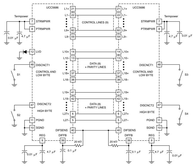
NOTE A: Close S1, S2, S3, and S4 to connect terminators in UCC5686. Open S1, S2, S3, and S4 to connect terminators in UCC5687.
