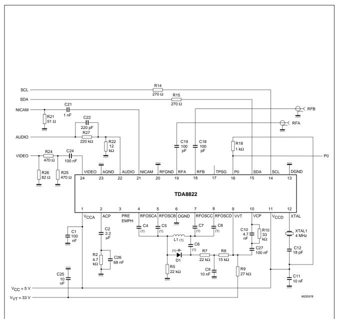
(1) The components marked: C4, C5, C6, C7, C8, L1 and D1 must be chosen from Table 11 to get the desired frequency range.
