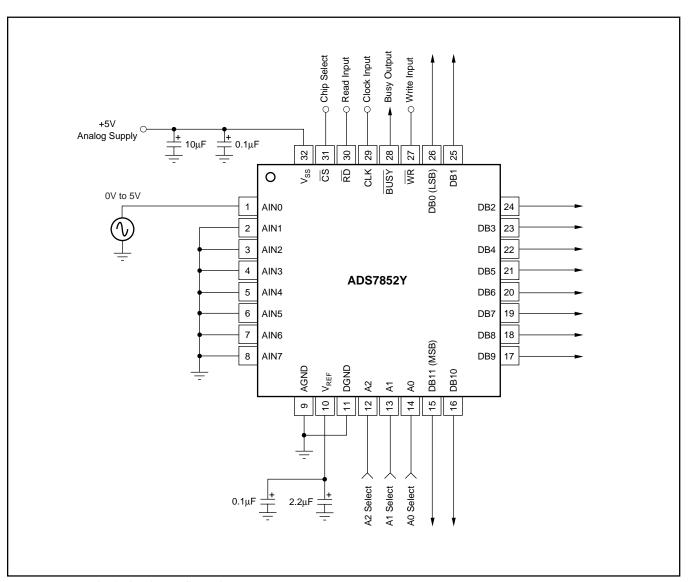
FIGURE 1. Typical Circuit Configuration.
