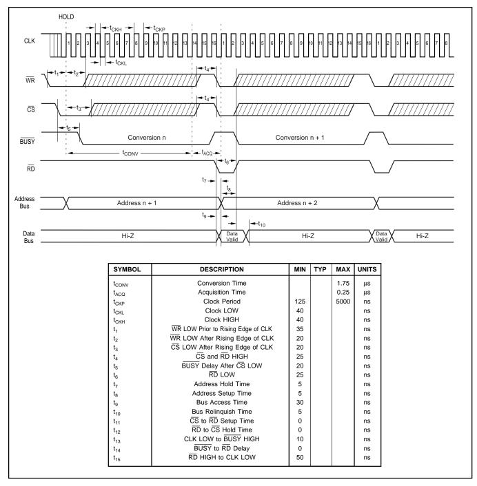
FIGURE 2. ADS7852 Write/Read Timing.
