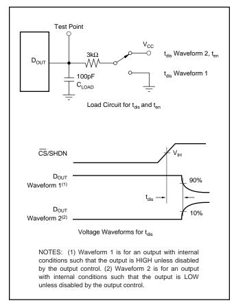
FIGURE 5. Timing Diagram and Test Circuits for Parameters in Figure 2.
