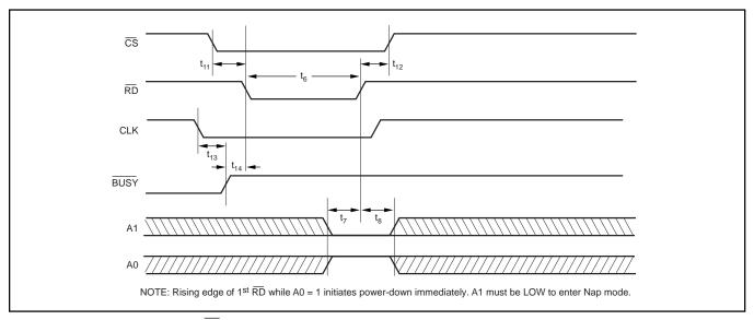
FIGURE 3. Entering Nap Using RD and A0.
