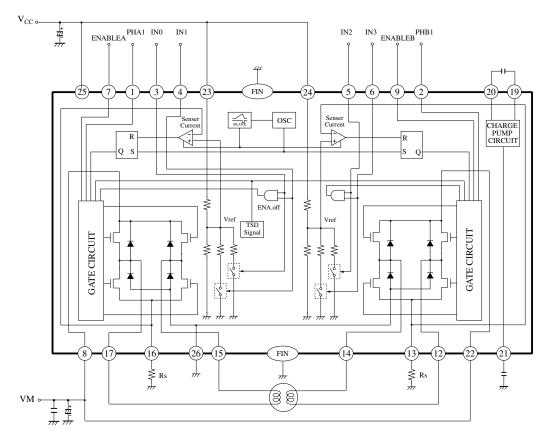
\* A voltage is applied externally to Terminals PHA1, PHB1, IN0 to 3, ENABLEA, ENABLEB, VREFA and VREFV, and may cause an overcurrent. To protect the device from overcurrent, insert an overcurrent protective resistor (1K $\Omega$  or over).
