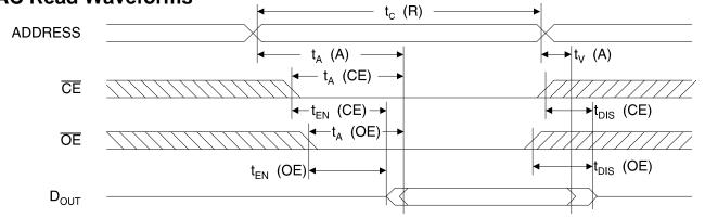
Notes: 1.  $\overline{\text{CE}}$  may be delayed up to  $t_{ACC}$  -  $t_{CE}$  after the address transition without impact on tACC.
