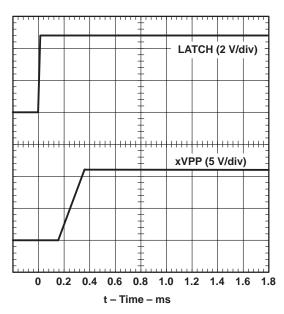
Figure 15. xVPP Propagation Delay and Rise Time With 1-μF Load, 12-V Switch
