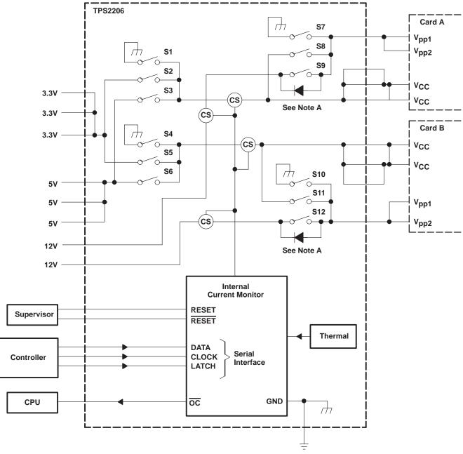
NOTE A: MOSFET switches S9 and S12 have a back-gate diode from the source to the drain. Unused switch inputs should never be grounded.
