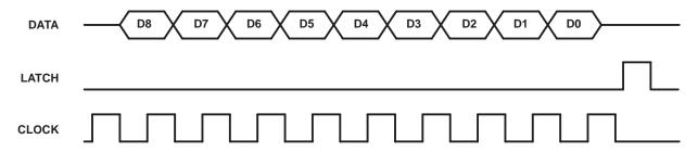
NOTE A: Data is clocked in on the positive leading edge of the clock. The latch should occur before the next positive leading edge of the clock. For definition of D0 to D8, see the control logic table.
