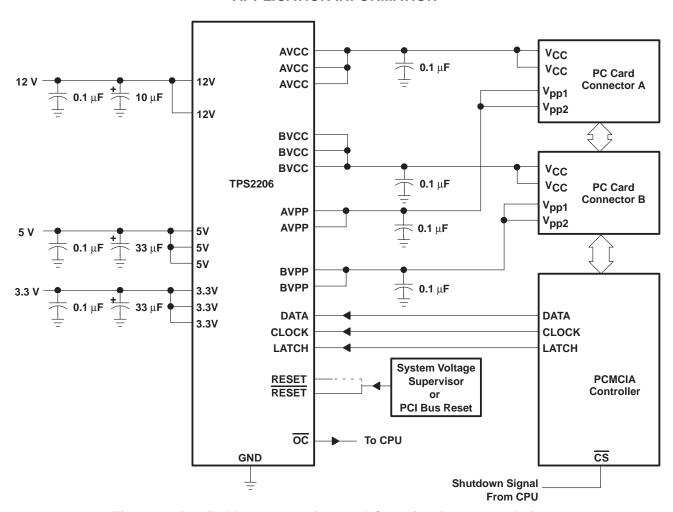
Figure 33. Detailed Interconnections and Capacitor Recommendations
