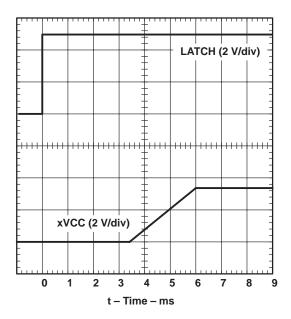
Figure 3. xVCC Propagation Delay and Rise Time With 1- $\mu$ F Load, 3.3-V Switch, (V<sub>I(5V)</sub> = 5 V)
