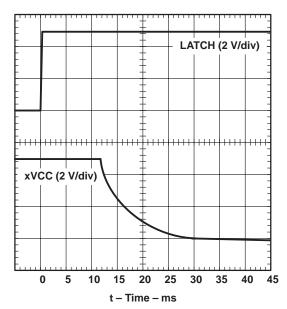
Figure 14. xVCC Propagation Delay and Fall Time With 150-μF Load, 5-V Switch
