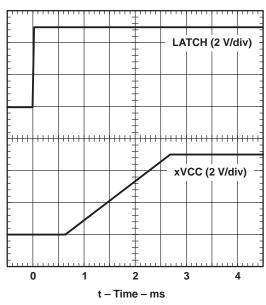
Figure 11. xVCC Propagation Delay and Rise Time With 1- $\mu$ F Load, 5-V Switch
