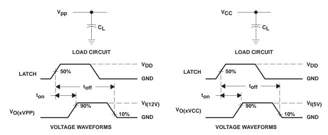
Figure 1. Test Circuits and Voltage Waveforms
