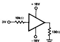
\* Oil Bath Burn-In: Use the oil bath heated to  $+125^{\circ}\text{C}$  to provide the heat sink necessary to maintain the junction temperature at  $< +175^{\circ}\text{C}$ .
