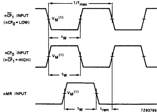
Fig.7 Waveforms showing removal time for nMR; minimum  $nCP_0$ ,  $n\overline{CP}_1$ , nMR pulse widths and maximum clock pulse frequency.
