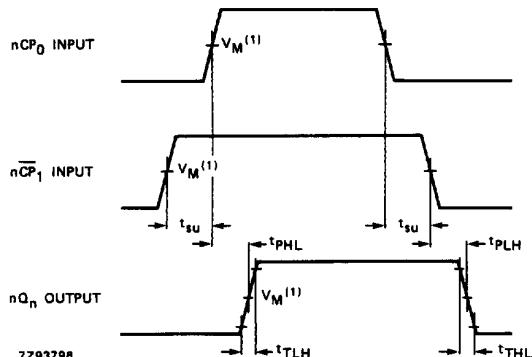
Fig.8 Waveforms showing set-up times for  $nCP_0$  to  $n\overline{CP}_1$  and  $n\overline{CP}_1$  to  $nCP_0$ , propagation delays and output transition times.
