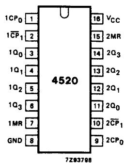
Fig.1 Pin configuration.
