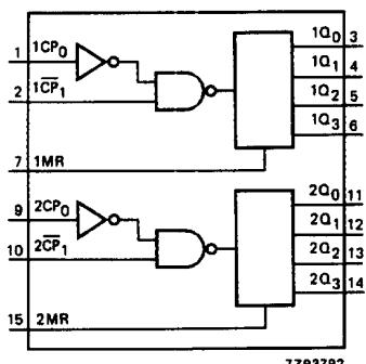
Fig.4 Functional diagram.
