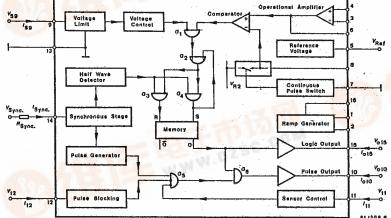
Fig. 1 Block diagram and pin connections
