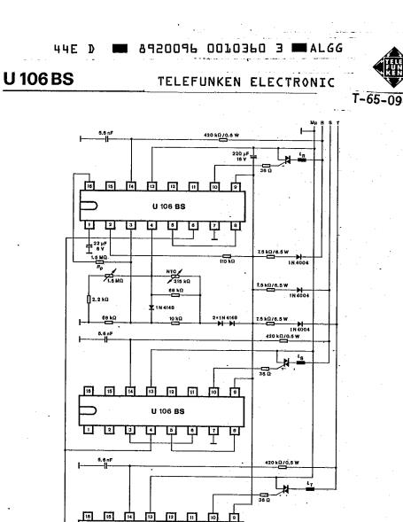
Fig. 25 Three-phase, two-point temperature control with superimposed proportional characteristic for a temperature range 60...280 °C
