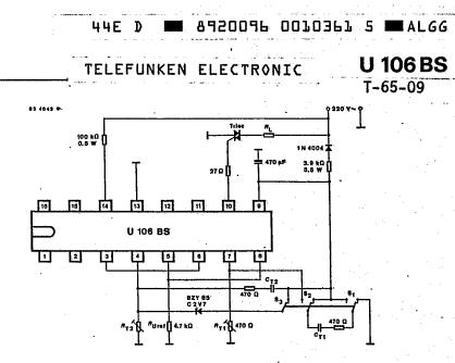
Fig. 26 One-shot switching delay circuit
