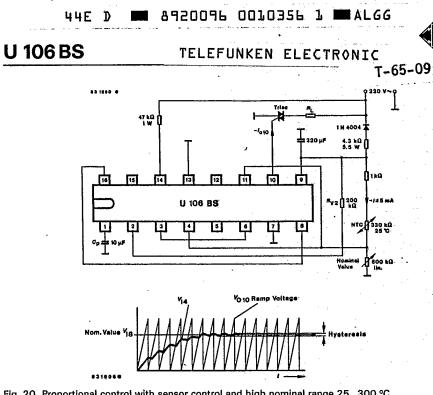
Fig. 20 Proportional control with sensor control and high nominal range 25...300 °C
