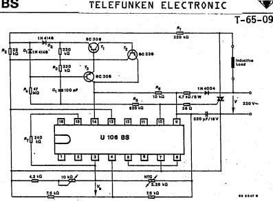
Fig. 23 Two-point temperature control circuit for inductive load
