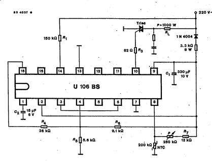
Fig. 24 Temperature control with superimposed proportional characteristic for a temperature range 30...110 °C and  $\pm$ 3 °C hysteresis.
