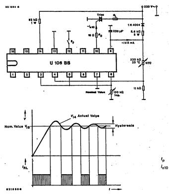
Fig. 19 Two point control with excessive temperature protection switch (S<sub>3</sub>) 60...150 °C.
