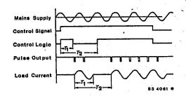
Fig. 27 Pulse diagram of a "one-shot" switching delay
