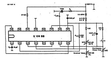
Fig. 21 Proportional control with adjustable continuous pulse circuit limiting boundary switch and transmission control
