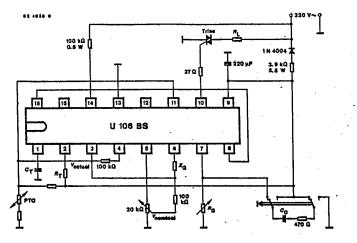
Fig. 17 Proportional controller with full-load switched-on
